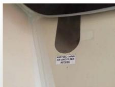
For 737-700IGW Aircraft equipped with a PATS Aircraft. 5-Cell Aft Tank installation under STC ST00936NY or ST01716NY, PATS has developed an Aft Bulkhead Maintenance Access Cover Product Improvement. This modification allows access to the AFT Master Fuel Cell Cabin Air Tube and Filter without disassembly of the AFT Barrier Bulkhead. This is a simple but effective product improvement to perform.
